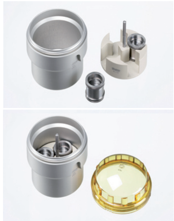
Carrier 4750 with lid 4751 and special accessories for determination of WHC.
