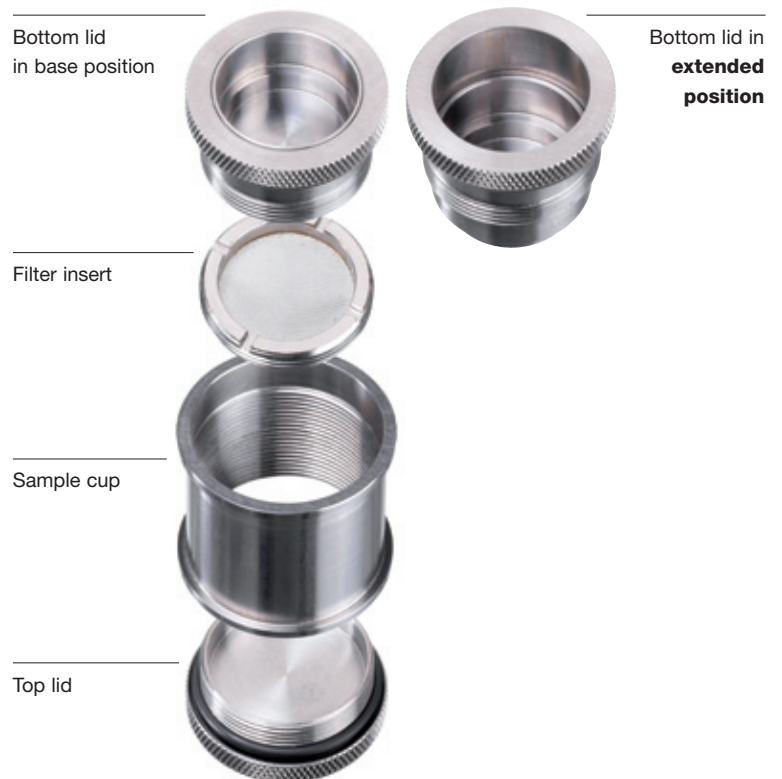
Fig. 1: Design of the sample cup
