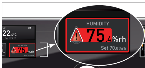
Fig. 22 Humidity monitoring triggered
