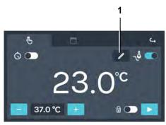
Fig. 73: 'Manual mode → Temperature drop → Editing'
