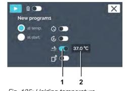
Fig. 135: Holding temperature
