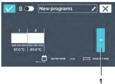
Fig. 114: Adding a program segment [New program segment] button
