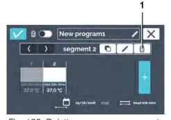
Fig. 122: Deleting a program segment 1 [Delete program segment] button
