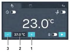
Fig. 85: 'Manual mode → Set temperature'
