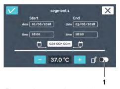
10. ▶ If an additional device is to be switched on in the interior or the ventilation opening is to be opened during the program segment, you can activate the control contact for it here.
