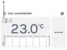
Fig. 59: Main screen, standstill mode, temperature guard active
