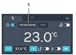
Fig. 68: 'Manual mode → Start delay → Start date'
