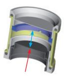
Fig. 4: Longitudinal section through the sample cup assembled for centrifugation
