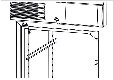
Fig. 210: Removing the support rails
