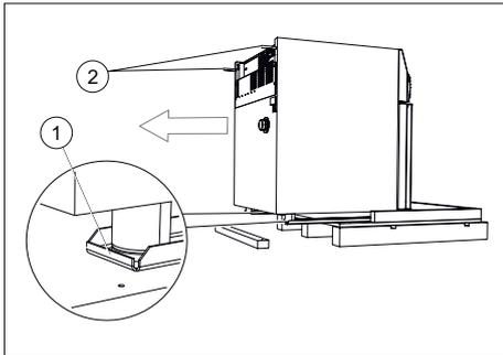
Fig. 25: Pulling incubator forward
