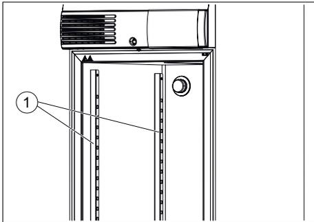
Fig. 213: Latching rails
