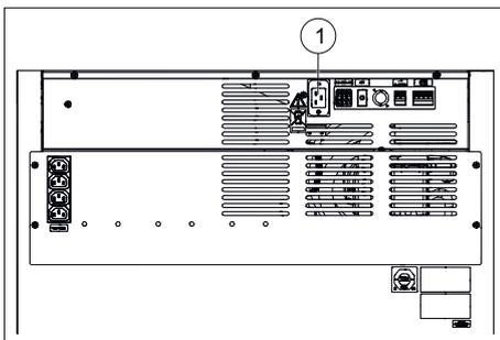
Fig. 27: Power supply connection
