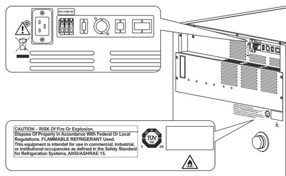
Fig. 3: Instructions on the rear side of the incubator
