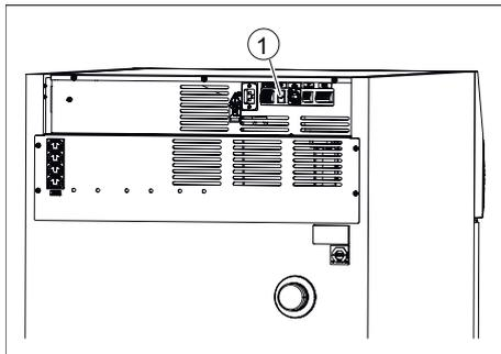
*Fig. 216: Activating the automatic circuit breaker*
