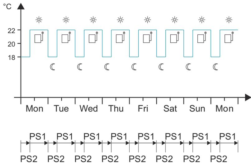
Fig. 229: Diagram 'External devices are integrated in program mode, e.g. DAY/NIGHT simulation.'
