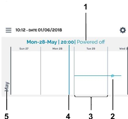
The display can be scrolled horizontally to the left and right. The dot on the display bar (4) shows the current position on the scale. Date, time and temperature of this time are displayed (1).
