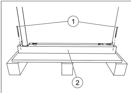
Fig. 17: Front wooden beam
