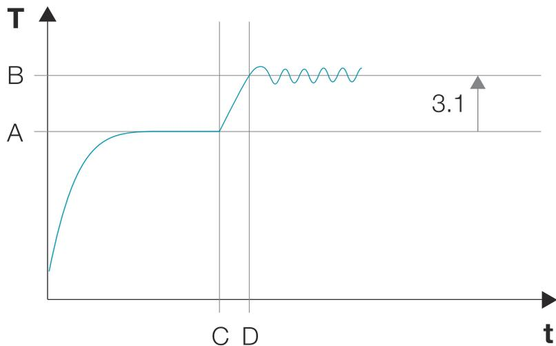
Fig. 155: Diagram of 'Temperature guard', class 3.1
