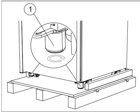
Fig. 20: Screwing in levelling elements
