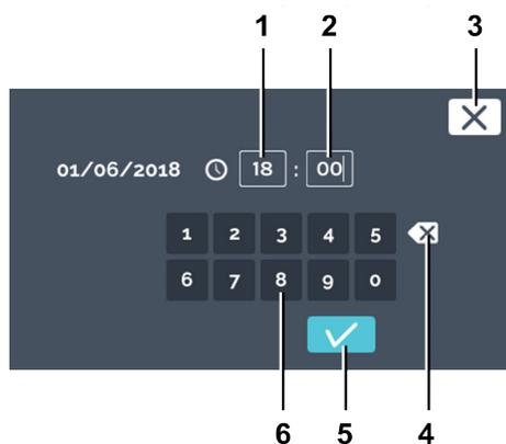
5. Enter the time. Confirm the input of the start time with the [Confirmation] button.
