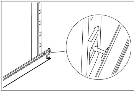
Fig. 44: Snapping telescopic rails in at the rear
