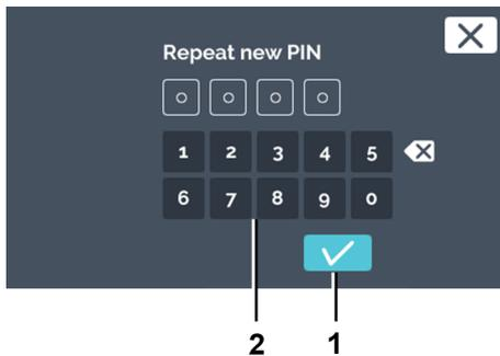
4. Enter the new admin PIN again via the keypad and confirm the input with the [Confirmation] button.
