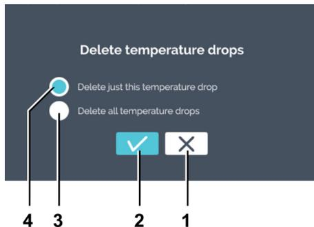
4. Select whether you would like to delete only the current temperature drop or all temperature drops. Confirm the selection with the *[Confirmation]* button.
