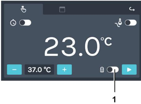
Fig. 82: 'Manual mode → PIN protection'
