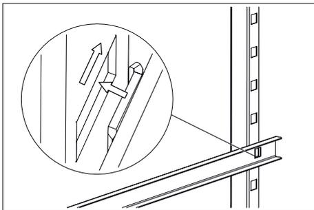
Fig. 41: Snapping in support rail at the rear
