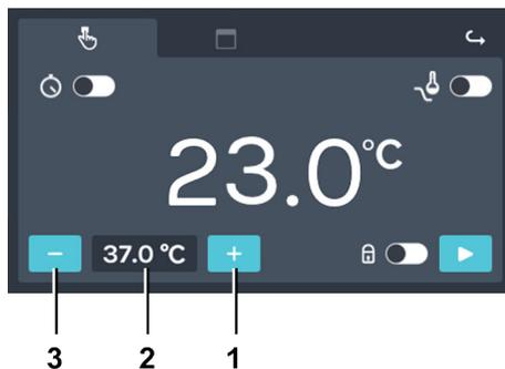
Fig. 85: 'Manual mode → Set temperature'
