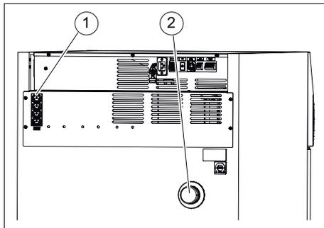
*Fig. 29: Connections for additional devices*
