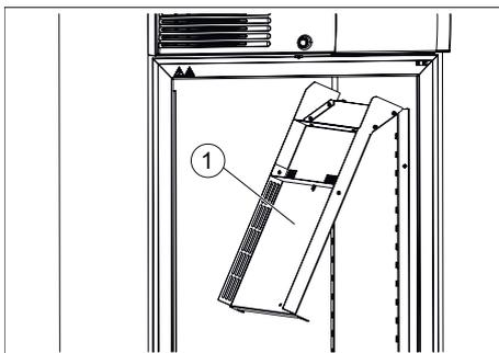
Fig. 212: Top baffle sheet
