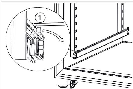
Fig. 49: Turning the telescopic rail, front side
