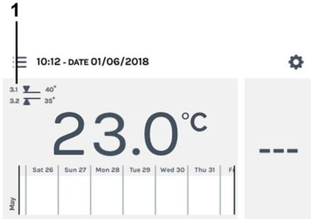
Fig. 59: Main screen, standstill mode, temperature guard active
