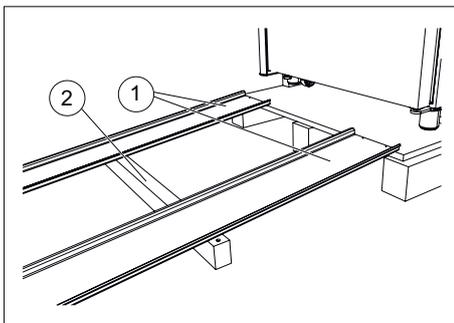
Fig. 19: Wooden beam under the metal rails
