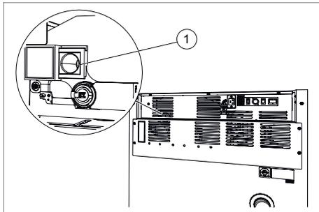
Fig. 164: Passive dehumidification ventilation opening
