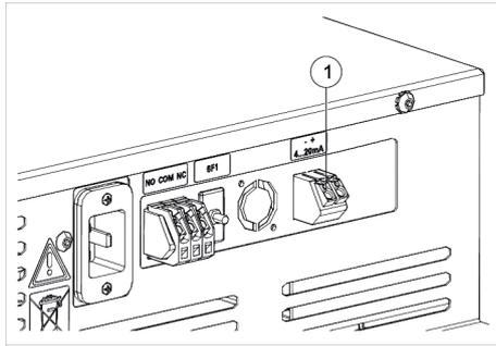
The device is equipped with an additional, independent PT 100 temperature sensor. The temperature values are output via a 4-20 mA analogue output on the rear side of the device.
