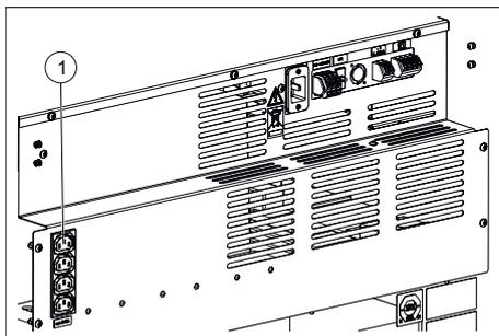
The incubator has a socket strip arranged on the rear side of the device. This socket strip can be switched on and off individually or time-controlled via the touchscreen. It is operated via the control contact function → *Chapter 6.12.6 'Control contact (option)' on page 103*. It is particularly meant for the operation of additional devices in the incubator.
