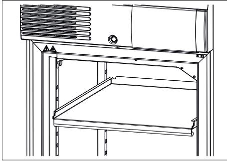
Fig. 209: Removing the slide-in module
