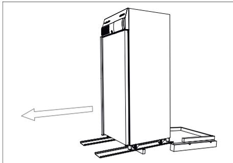
Fig. 21: Rolling the incubator down over metal rails
